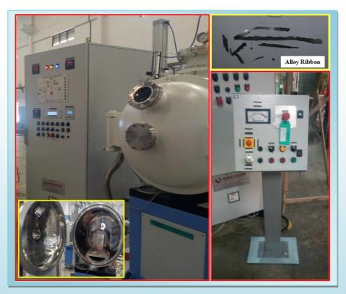
Installation of New Facility in TRC: Vacuum RF Induction Furnace/Melt Spinning Unit for Alloy Preparation (May 21, 2018). Supplier: VACUUM TECHNIQUES PVT. LTD, Bangalore Melt Capacity: 2 to 12 gm. Advanced Facility for Rapid Solidification of Metallic Alloys
